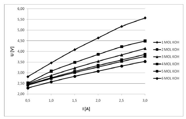
Fig. 1 - Measurements on elektrolyzer with different KOH solutions
